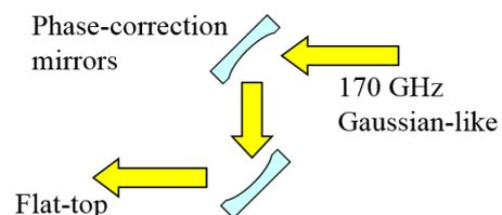
**Fig.2** Schematic of a beam profile conversion system.
