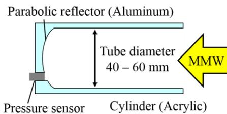
Fig.4 Schematic of breakdown and pressure measurement system.
