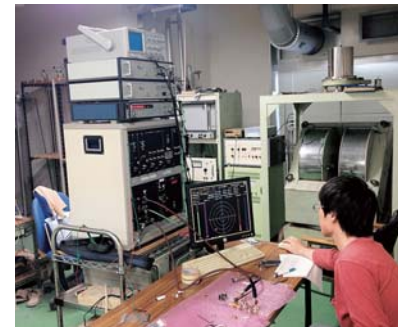
mm-wave vector network analyzer (MVNA)
