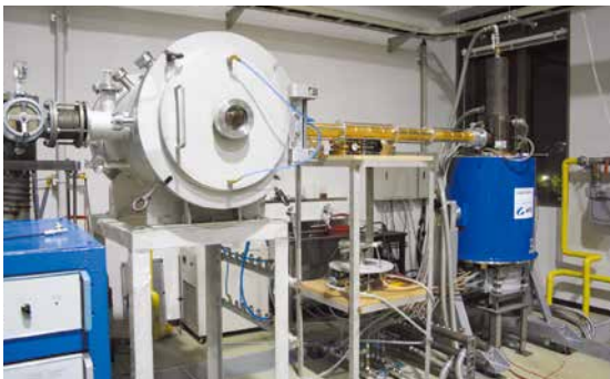
The world's first 300 GHz/2.3 kW high-power electromagnetic wave irradiation system
