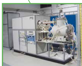
28-GHz microwave sintering system (Room 101)
