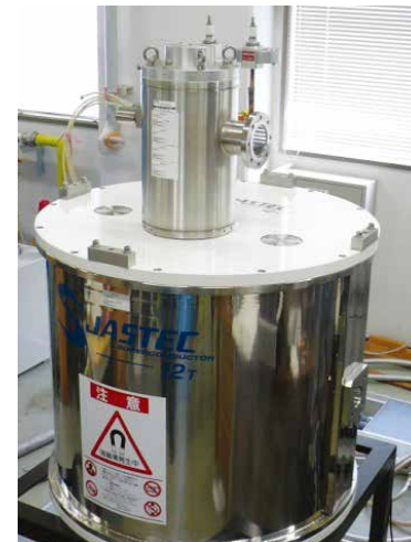
A high-power pulse gyrotron mounted on a 12-T SC magnet is under development for use on LHD in the National Institute for Fusion Science.
