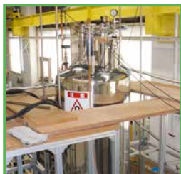
1 THz gyrotron FU CW III with a 20-T superconducting magnet
