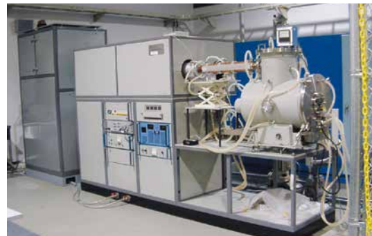
28 GHz/15 kW high-power electromagnetic wave irradiation system
