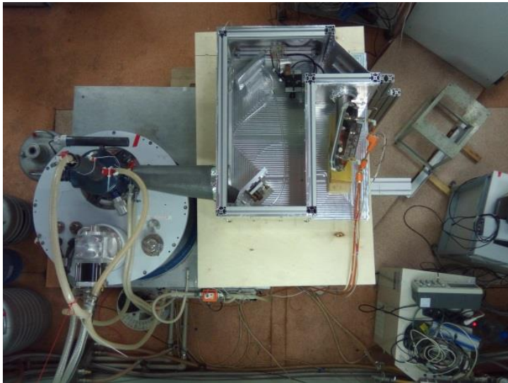
Fig. 2. Shielded box design for focusing the radiation on the fundamental frequency (gyrotron part on the left side).
