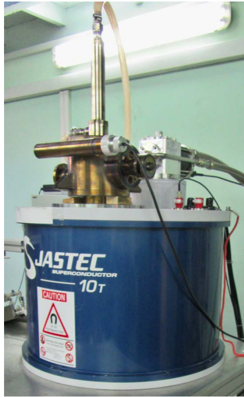
Fig. 1. Photo of the gyrotron and an experimental setup with the tube inside a cryomagnet.
