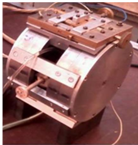
Fig.1 THz CW clinotron tubes packaged in compact 1 T focusing systems
