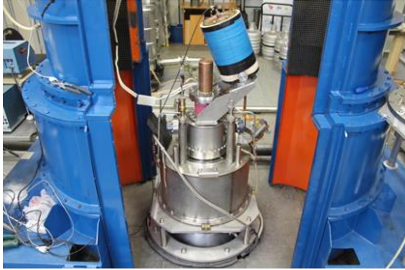
Photo of the relativistic gyrotron, installed on the experimental stand "Saturn-F"
