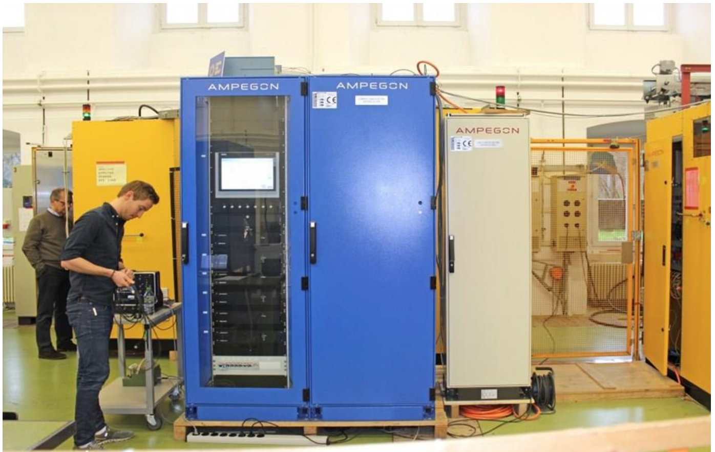
Factory acceptance tests of the high-voltage power supply systems ( image courtesy to ITER)
